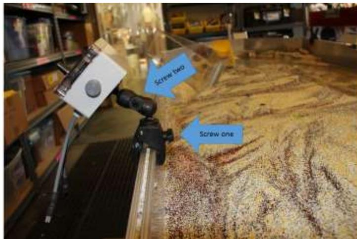
**Be sure the controller claw bracket is secure along the inside edge of the box by tightening Screw One. Screw Two allows for the removal of the Alix controller box.**
