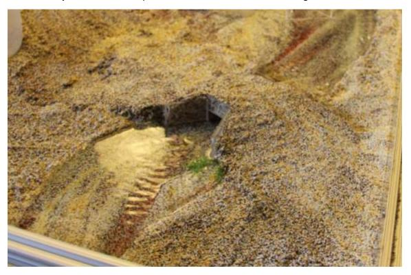
Either way, some things to look for when the flow exceeds the capability of the culvert include erosion and scouring.
