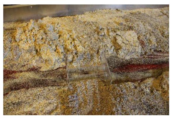
Double culverts double the wetted perimeter of the culvert and allow for larger flows.
