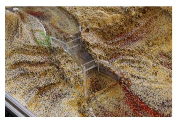
To use a culvert, place it in line with the stream flow. Next, push the media along the sides of the culvert so that the water is flowing into it.
