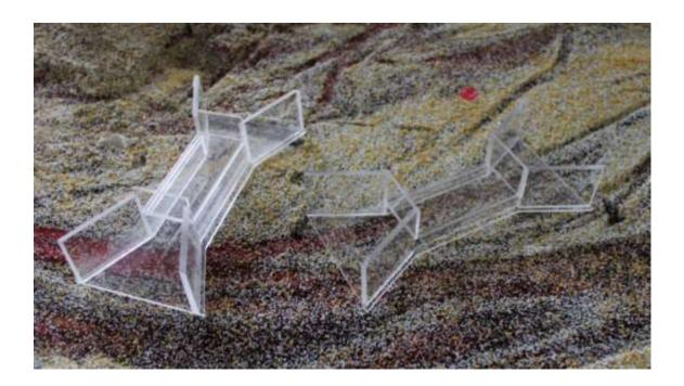
The culverts are clear so that one can see how the sediment flows through them.
