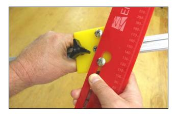
3. Fit the same opening over the head of the top bolt and release the spring.
