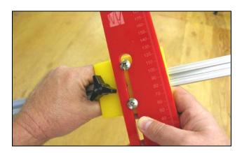
To survey points within the model, set up your laser (not included with Academic Kit) so that the beam is about 10 cm above the upper edge of the box. Be sure that you can see the beam when standing at the corners of the box and that the beam crosses the level rod at the highest and lowest points to be surveyed.
