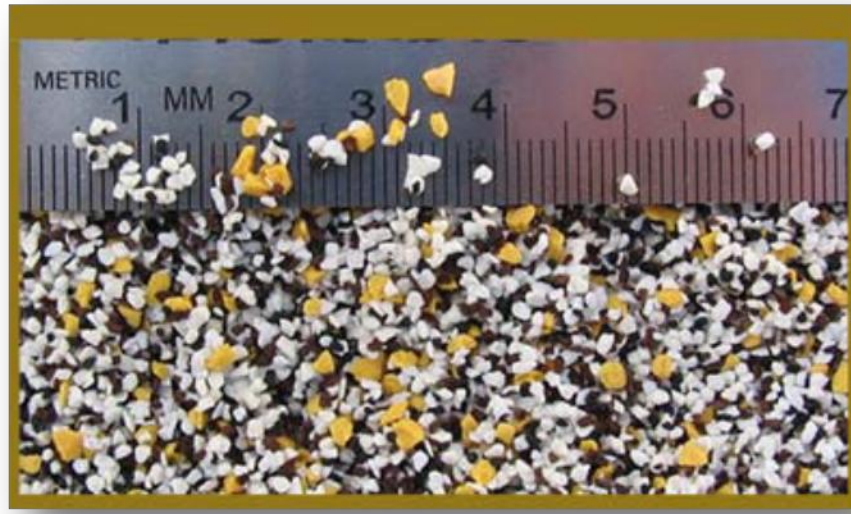
Figure 3.2: Photograph of the Coded by Size Thermoset Plastic Media
