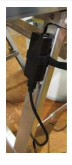
12-volt power supply with Ground Fault Circuit Interrupter, input standard 115-volt, 60Hz. Export models shipped with appropriate CE-approved power supply and connectors.
