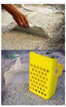
Two scrapers for moving and shaping media. Two large scoops: one perforated and one non-perforated
