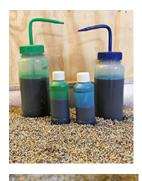
Concentrated blue and green dye with injection bottles for flow visualization
