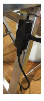
12-volt power supply with Ground Fault Circuit Interrupter, input standard 115-volt, 60Hz. Export models shipped with appropriate CE-approved power supply and connectors.
