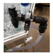
Water flows from upstream reservoir through Inlet Pipe to the acrylic Energy Dissipater Unit (EDU)
