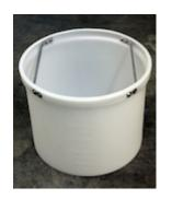
Two 27 gal. (110 L) polypropylene reservoirs, graduated, with supports on downstream reservoir for sediment filter
