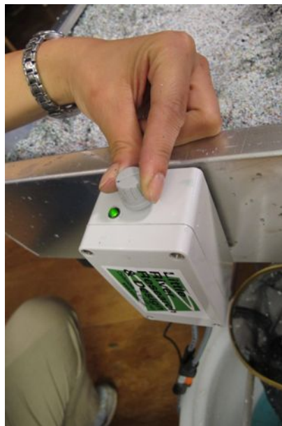
Turn the knob on the controller clockwise to increase flow and counterclockwise to decrease flow.
