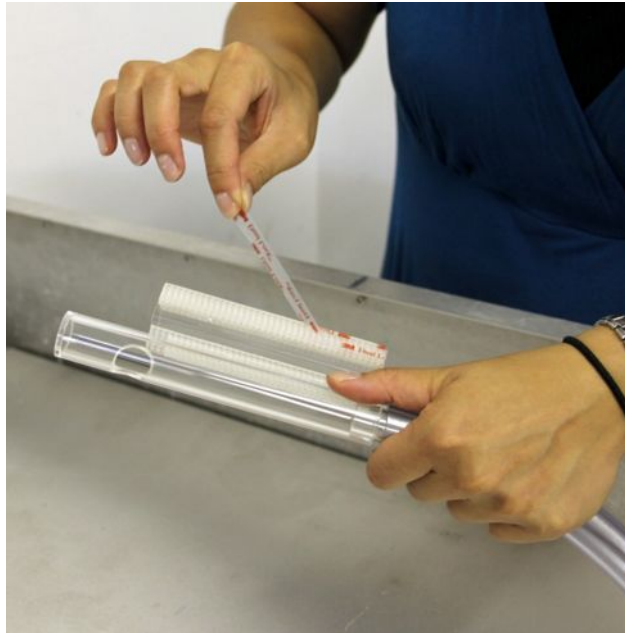
Peel the backing off of the adhesive on the mushroom fasteners.
