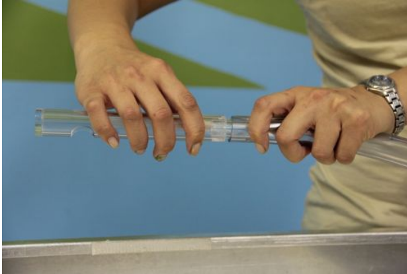
Connect the flow outlet and tubing.
