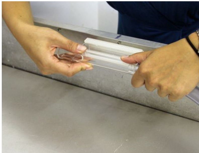
Attach the flow outlet to the upstream end of the box using the mushroom fasteners and the outlet mount.
