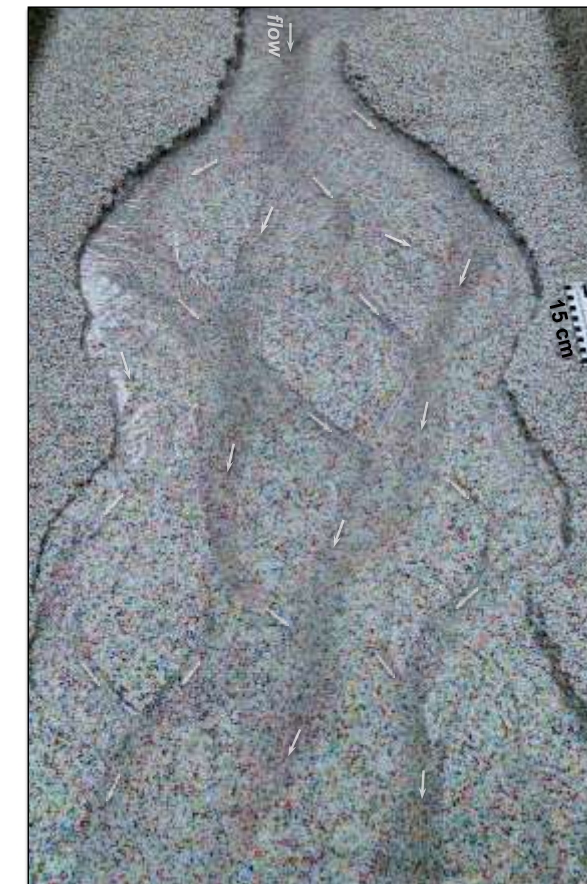
Example of a braided channel developed in the model. Discharge was 88 \times 10^{-6} \text{ m}^3 \text{ s}^{-1} and the slope was 0.030. Run time was 15 min. Arrows indicate some of the active channels.
