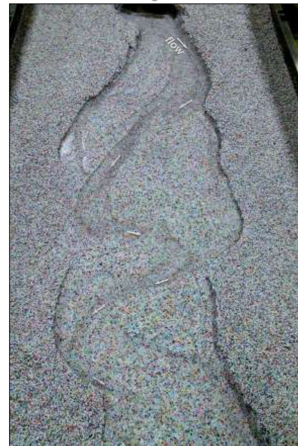
Example of a meandering channel developed in the model. Discharge was 50 \times 10^{-6} \text{ m}^3 \text{ s}^{-1} and the slope was 0.034. Run time was 30 min. Arrows indicate the active channel. Scale is the same as in the photo to the right.
