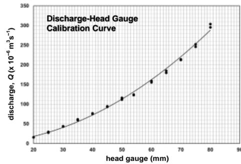
Prior to conducting the experiments, discharge was measured by collecting water from the standpipe for a given amount of time. Discharge was measured under various flow settings and head gauge elevations to calibrate discharge with the head gauge reading.
