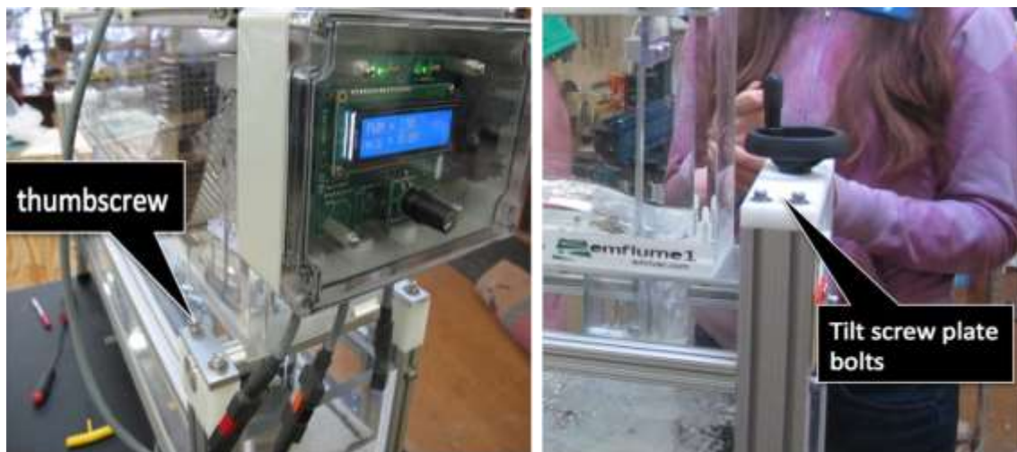
Figure 4-1 upstream thumb screw and downstream tilt
