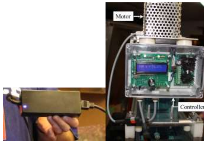
Figure 3-4 Power supply adapter, flow controller and motor
