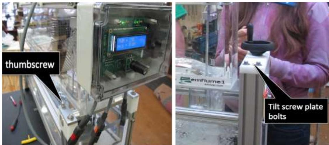
Figure 4-1 upstream thumb screw and downstream tilt
