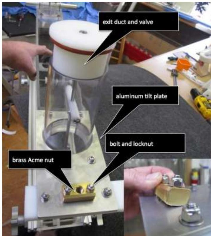
Figure 3-7 Underside of the downstream end of the Emflume1. The brass Acme nut is threaded onto the tilt screw (not shown). **Do not alter the tightness of the bolts attaching this nut to the aluminum plate.** They are secured by locknuts and intentionally left loose to allow for up and down movement of the flume using the tilt crank.
