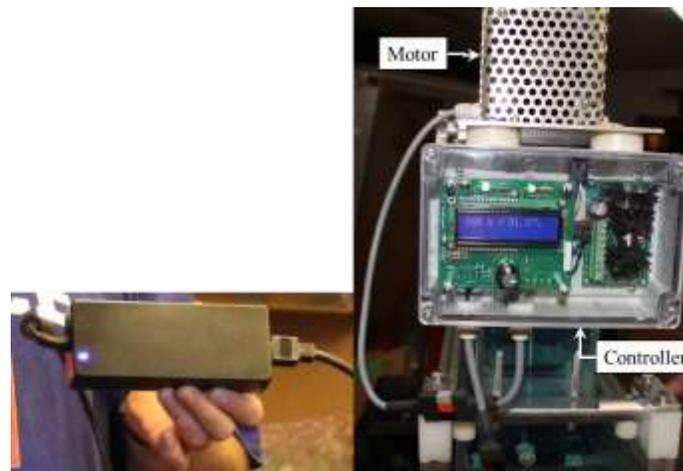
Figure 3-4 Power supply adapter, flow controller and motor
