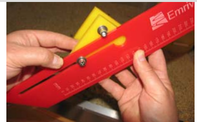
3 - Slide rod up and over bolt head -
