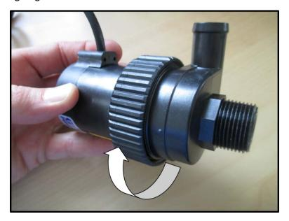
3. Pull threaded portion of pump housing to remove. Be careful not to remove the O-ring.
