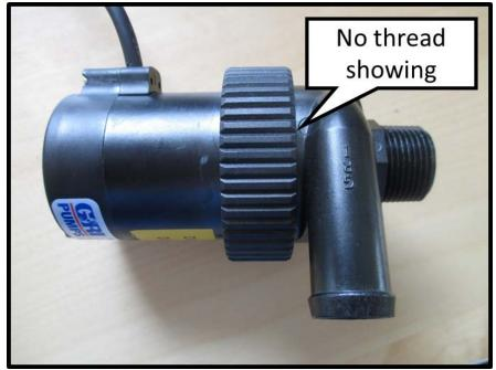
7. Attach filter and tubing. Submerge pump fully before restarting. Agitating the assembly lightly in the water will help clear air from the filter and pump.
