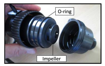
4. Remove the impeller by pulling it from the pump housing.
