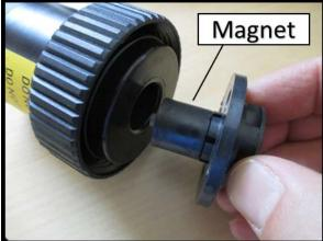
5. Clean all parts by rinsing with water. Make sure the narrow gaps around the impeller are clear of debris.
