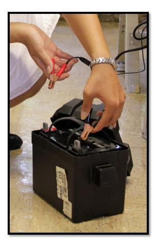
Attach the alligator clips on the battery adapter to the terminals on the battery. Connect the negative (black) clip to the negative terminal, and the positive (red) clip to the positive battery terminal. Be careful not to switch the positive and negative!
