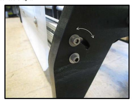
To extend the baffle, loosen the button cap screws on the rail (just slightly), with a 5/32" hex driver. Slide the perforated baffle down and retighten the screws.
