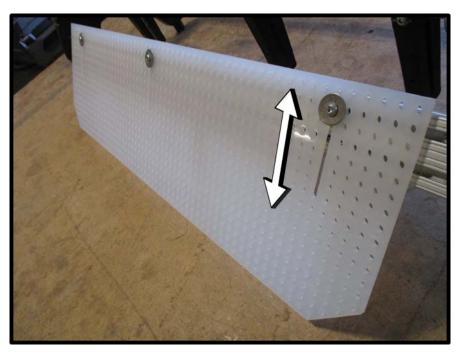
The paddle depth can be adjusted by loosening the lower screws on the black paddle clamps and sliding the clear paddle up or down.
