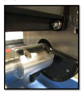
2. Position the paddle so it's plumb, hanging straight down from the shaft. Turn the timing pulley by hand until the magnet lines up with the sensor as show.
