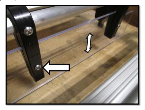
You may wish to experiment with the tilt of your model to maximize the body of water on the downstream end. NOTE: If you have a static model, you may shim the downstream end to lift it, but do not do this with the model fully loaded with water and media. This could risk personal injury or damage to the box. Make the adjustment with the box mostly empty and dry.
