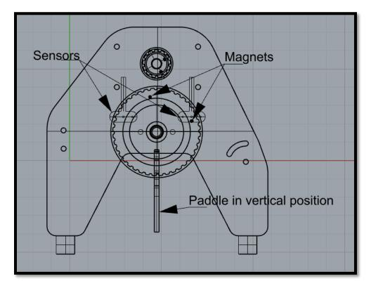
If the sensors and paddle do not appear properly aligned, reposition using the following steps.
