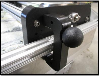
Adjust the angle of the 1"x2" rail by loosening the socket head bolts on both ends with a 3/16" hex driver. Pivot the rail. Start around  $45^{\circ}$ . Once in position, tighten the bolts. They only need to be snug, do not over tighten.
