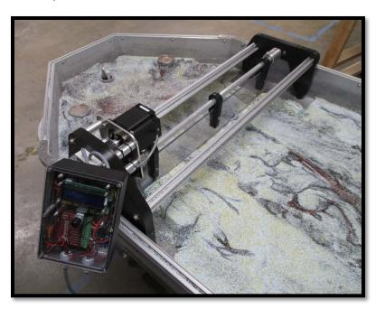
After placing the wavemaker into your Emriver table, secure the end opposite the motor end of the wavemaker to the side rail by inserting the  $\frac{1}{2}$ " rod with the black knob through the black plastic clamp into the threaded hole on the end plate.
