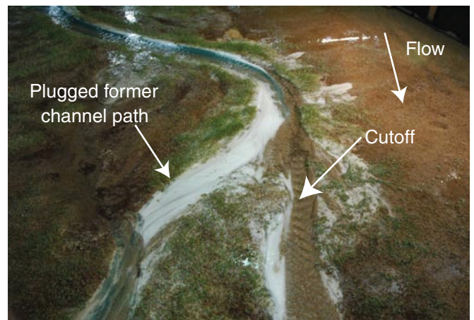
Fig. 5. Photograph of cutoff channel and fine sediment filling the former channel. Sediment colors are the same as Fig. 3. Fines also comprised the downstream end of the bar visible in the photograph. This was the final cutoff of the experiments and was caused by headward erosion rather than bar migration into a chute.
