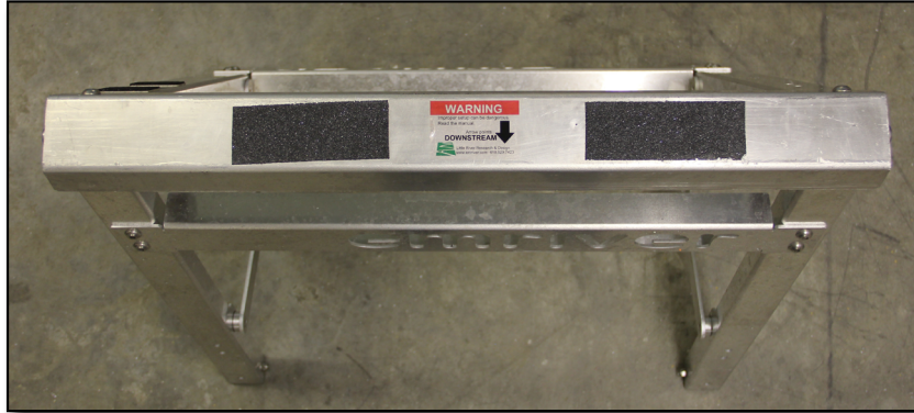
Figure 3. Labels on the supports indicate proper orientation, with the shorter support at the downstream end
