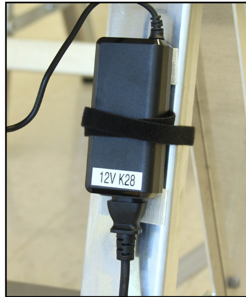
Figure 17. The DC power supply secured to the leg of the upstream support
