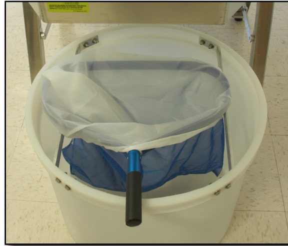
Figure 14. Place the sediment trap on the aluminum struts in the reservoir.
