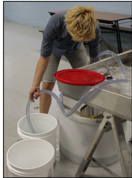
Figure 22. The controller and pump can be used to empty the reservoirs into media buckets.
