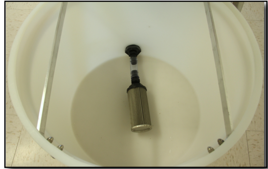
Figure 8. The downstream reservoir has a filter and struts for the sediment trap.
