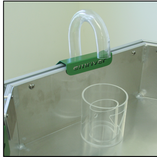
Figure 15. The EDU sits under the flow outlet with the V-notch pointing toward the downstream end of the box.
