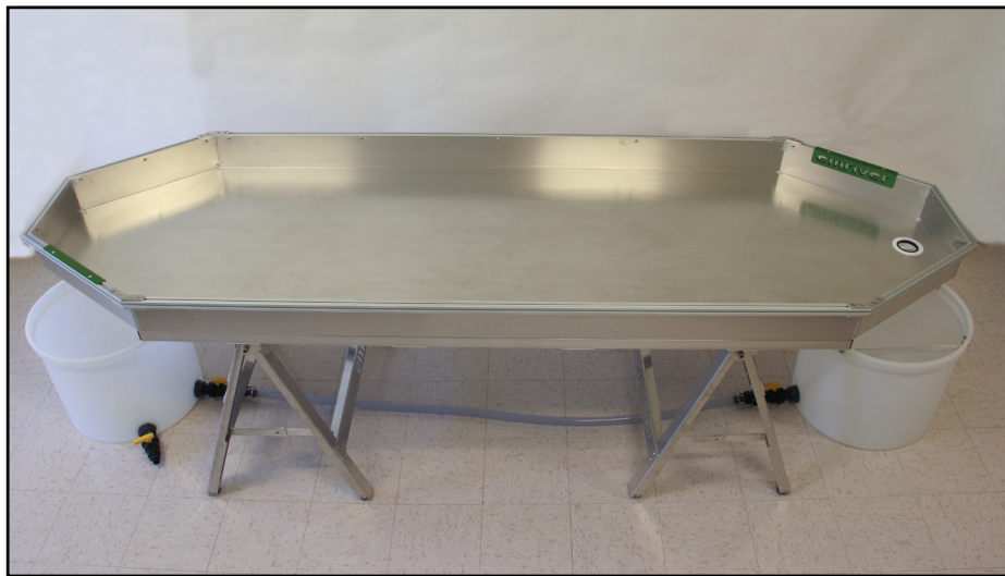
Figure 10. The Em3 box on the supports with upstream (L) and downstream (R) reservoirs positioned and the reservoir tubing connected
