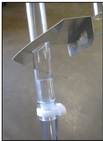
Figure 12. Pump tubing connected to the flow outlet
