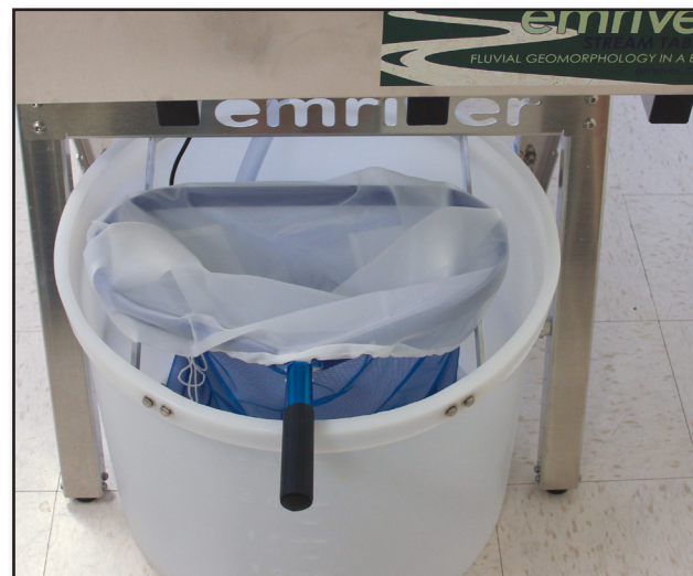
Figure 13. Place the sediment trap with the filter bag insert on the reservoir bars.
