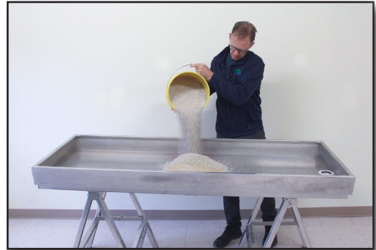
Figure 18. Pour the media into the box.
