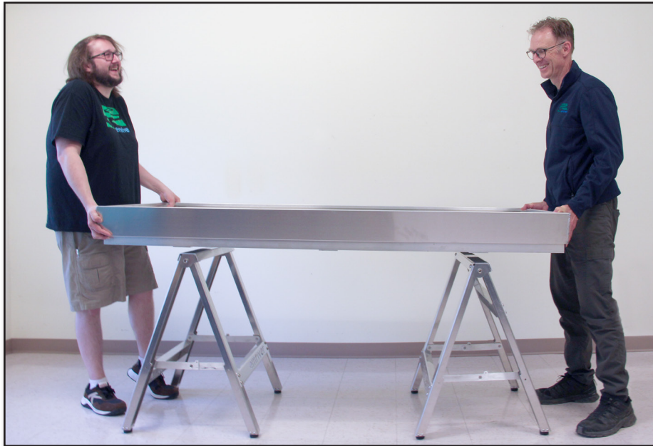
Figure 8. Place the box on the supports so the ribs rest on the support tops. It's easier with two people.
