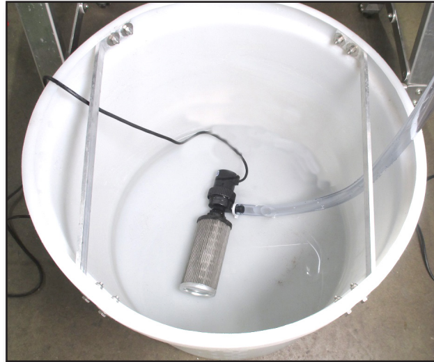
Figure 12. Place the pump with filter in the bottom of the reservoir, lying on its side.
