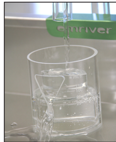
Figure 27. The EDU showing about 25ml/sec flow rate.
