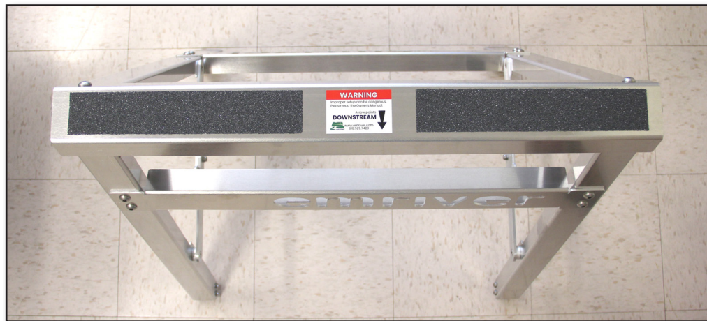
Figure 6. Labels on the supports indicate proper orientation, with the shorter support at the downstream end.
