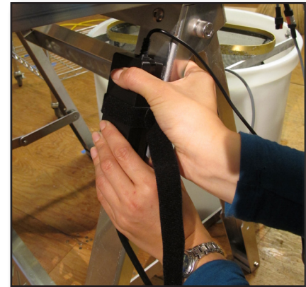
Figure 19. Attach the DC power supply to the leg of the upstream support.
