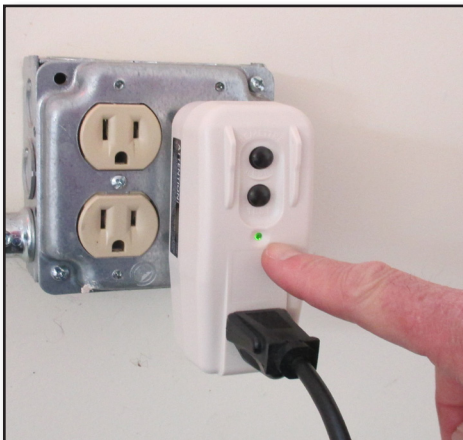
Figure 20. The green light on the GFCI indicates the circuit is protected.
