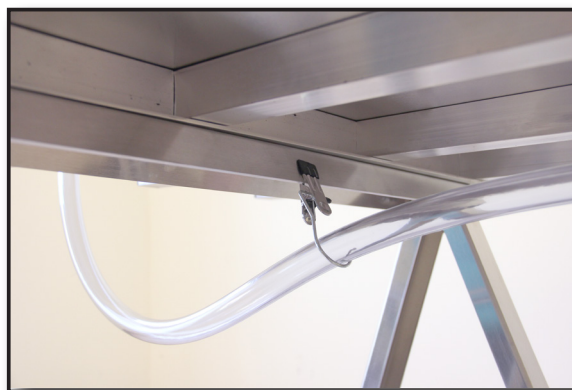
Figure 14. Hang the flexible tubing from the supports with the hanger clips.
