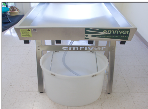
Figure 11. Place the reservoir beneath the support at the downstream end.
