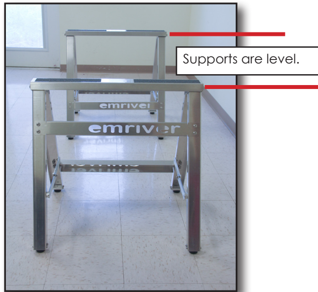
Figure 5. Look from the end to ensure the supports are level with each other.
