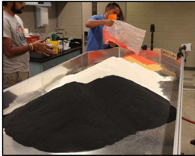
Figure 5.1 Unmixed media in the Em4 box.
