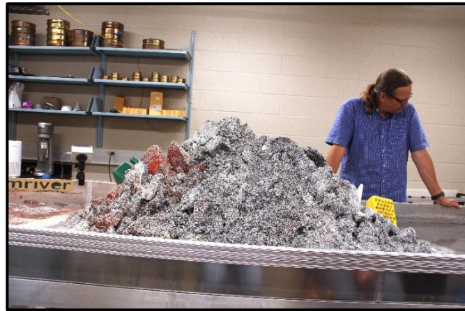
Figure 10.1 Pile up the media to aid drainage.
