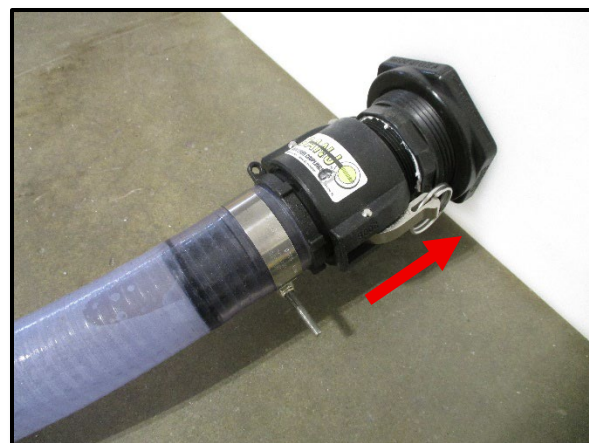
Figure 2.5 Push the levers toward the reservoir.
