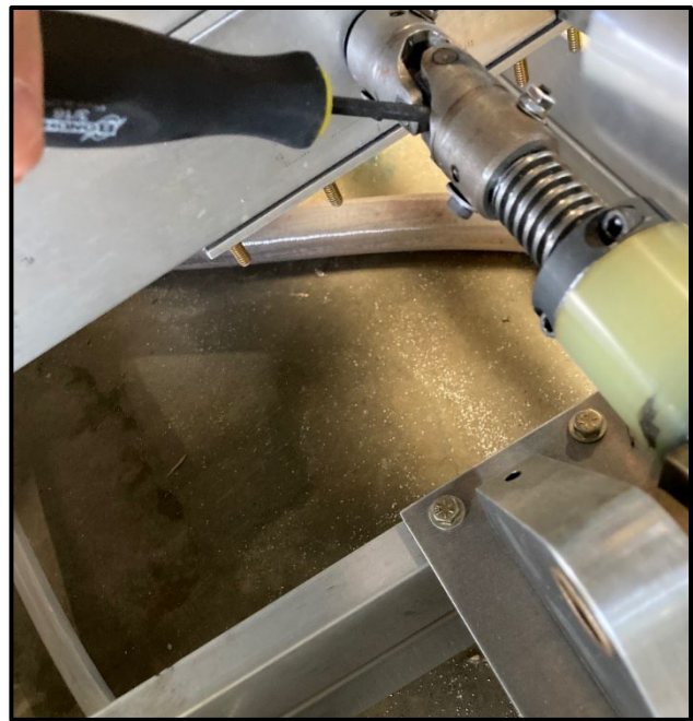
Figure 12.2 Insert the screwdriver through the U-Joint.
