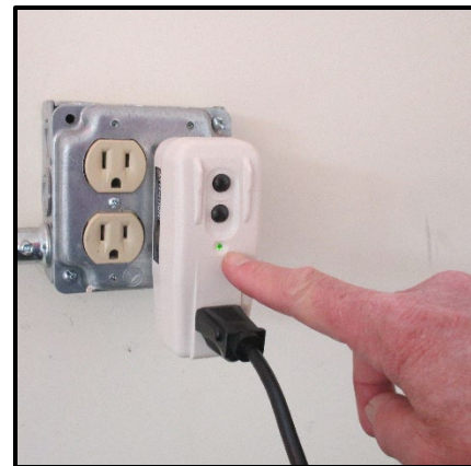
Figure 9.1 A green light indicates the GFCI is working correctly.
